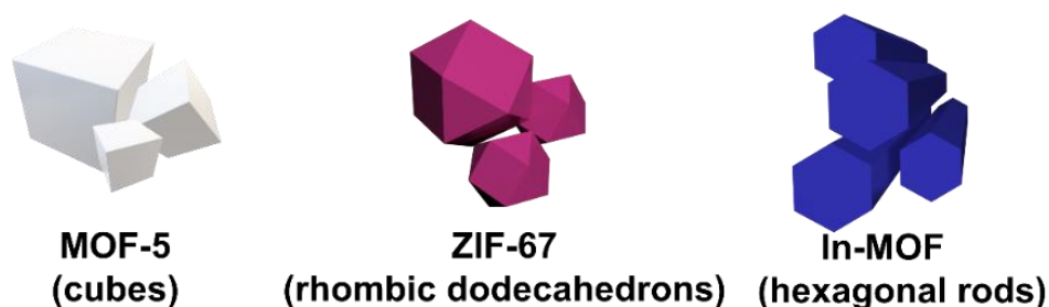
Figure 10. Three different MOF structures: cubes (MOF-5), rhombic dodecahedrons (ZIF-67) and hexagon rods (In-MOF).
