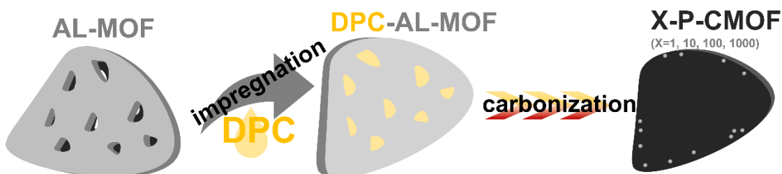
Figure 35. Schematic representation of 1,10,100,1000-P-CMOF synthesis.
