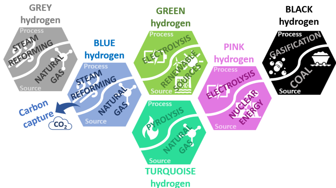
Figure 1. Different types of hydrogen based on the process and source of its production.
