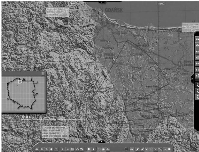
Screenshot 7.5. Effects of terrain elevation and obstacles on radar coverage.
