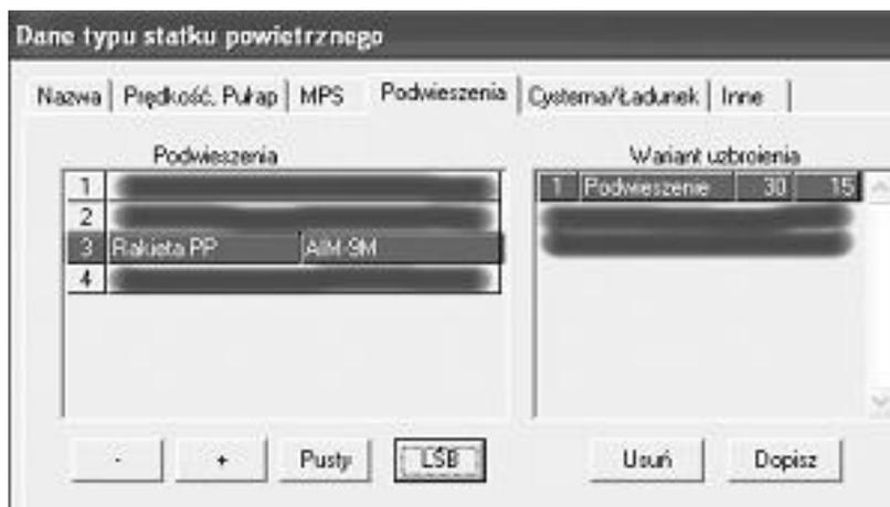
Screenshot 7.1. A user interface example – Aircraft tactical and technical characteristics form with COMBAT PAYLOAD data opened to add air to air missile AIM-9M.
