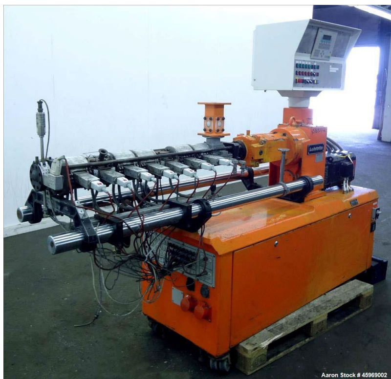
Fig. 1. Twin-screw extruder Model LSM34GL from Leistritz Inc. (Germany)
