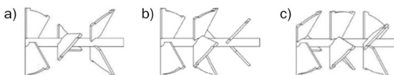
Fig. 1. Sketch of tested new geometries of mixing inserts: variant a), b), c)
