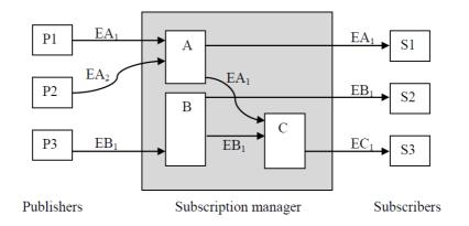
Figure 8.2. Implicit invocations with publish-subscribe mechanism. Publishers generate events *A* and *B* type. Communication hub generates event of *C* type after receiving *A* and *B* type. Subscribers *S1*, *S2*, *S3* are subscribed on events *A*, *B*, *C* accordingly.
