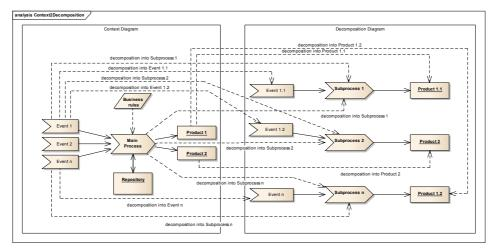
Figure 5.3. Rules for mapping a context diagram onto a process decomposition diagram.
