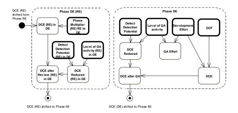
Figure 1.4. Model structure for design phase (DE) [SRGR13b].
