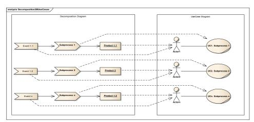
Figure 5.4. Rules of mapping process decomposition diagram onto BUC diagram.
