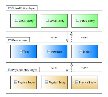
Figure 8.3. Layers pattern in IoT example.
