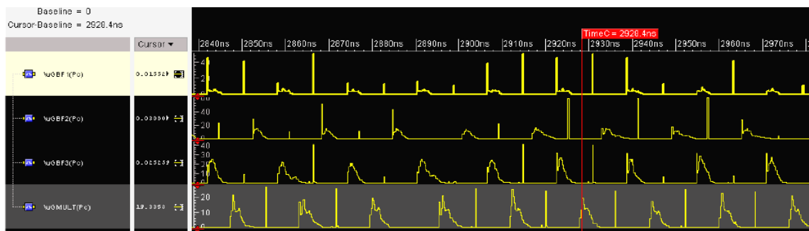
Figure 2.20. Current profiles of four synchronous GALS FFT blocks with phase modulation [22]
